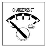
The CHARGE/ASSIST gage displays the charge (current) into and out of the hybrid battery.
